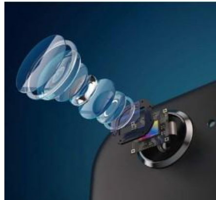
* Illustration of smartphone camera module structure
